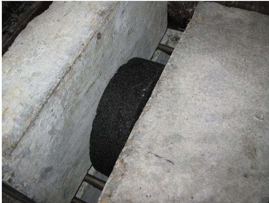
Figure 3.23 The HMA sample between lower and upper concrete blocks
