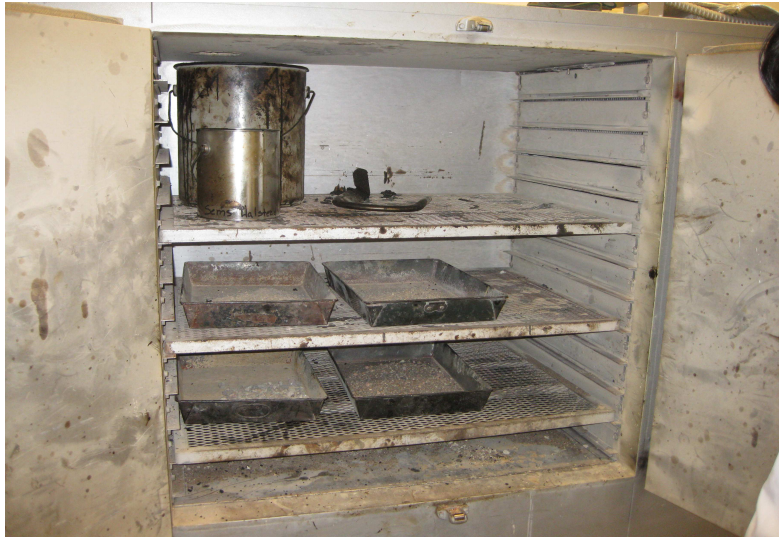
Figure 3.9 Heating of materials and binder to reach desired temperature
