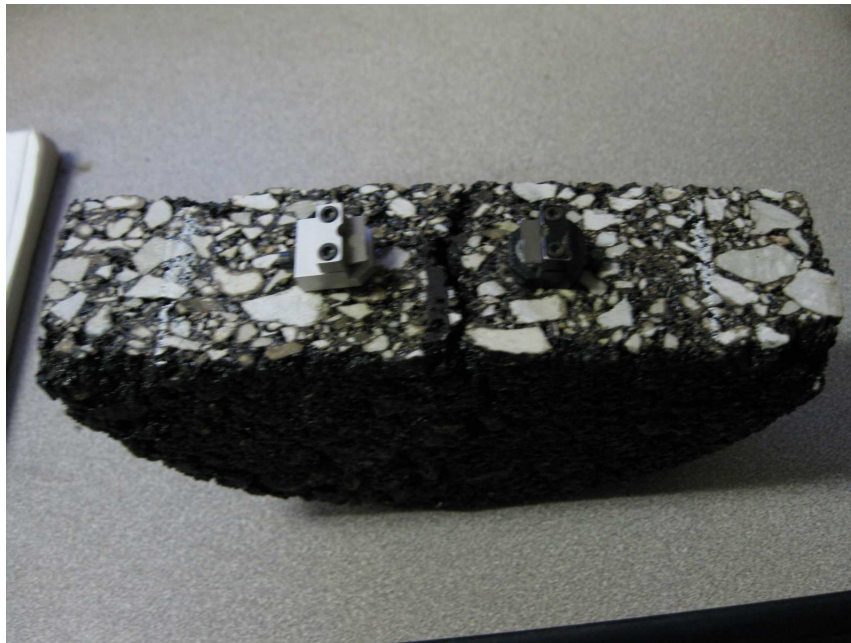
Figure 3.26. Appearance of a failed sample after testing
